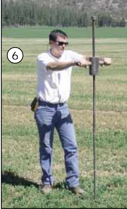
Figure 6. This steel rod is pounded into the soil to create a hole slightly larger than the diameter of the sensor. A coring device can also be used. Direct contact between the sensor and the soil is essential for reliable soil moisture readings.
