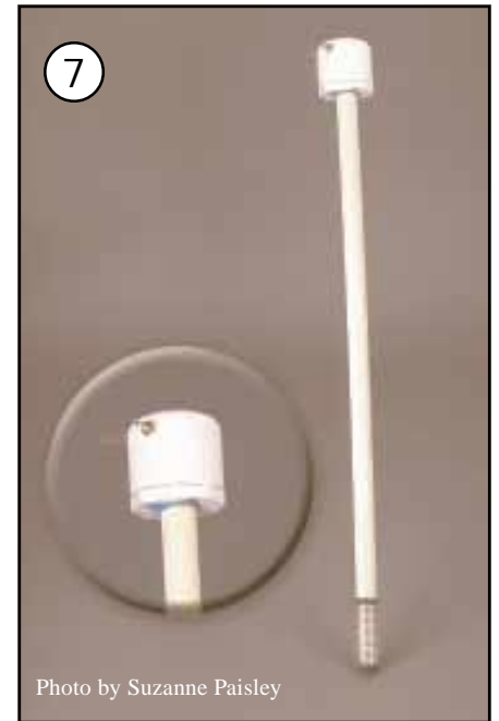
Figure 7. Soil moisture sensors can be glued to the end of PVC pipe. Wire leads from the sensor are connected to bolts protruding from a PVC cap for easy access while taking readings. This installation allows the sensors to be retrieved and reused.
